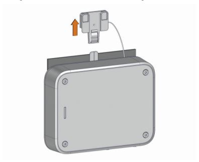
2 Press the tab 1 on the mounting bracket, and lift up 2 on the amplifier to disconnect it from the mount 3.
