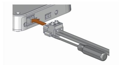
6 Using a 5 mm  $(^{7}/_{32}$  in.) flat (slotted) screwdriver, secure the power terminal block to the amplifier.
